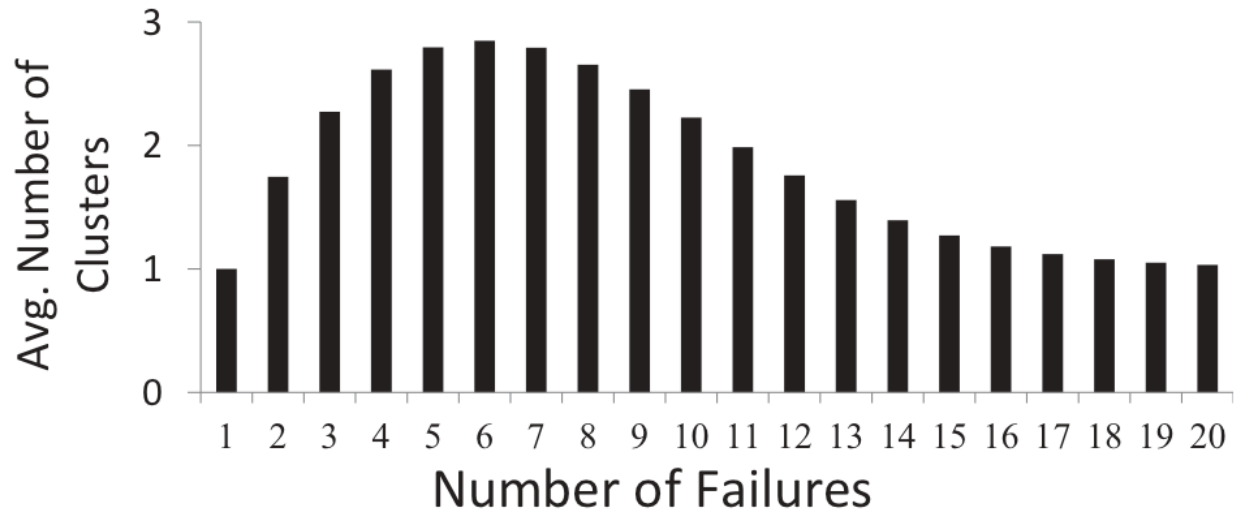
Figure 3: The average number of clusters versus the number of failures for CORE's code parameters (14,12,5)
