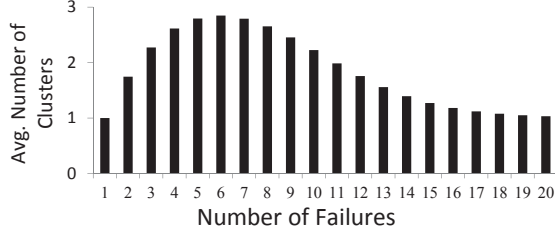
Figure 3: The average number of clusters versus the number of failures for CORE's code parameters (14,12,5)
