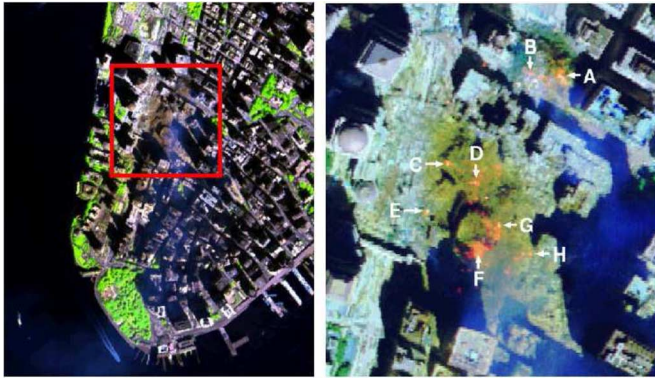
Fig. 6. False color composition of an AVIRIS hyperspectral image collected by NASA's Jet Propulsion Laboratory over lower Manhattan on Sept. 16, 2001 (left). Location of thermal hot spots in the fires observed in World Trade Center area, available online: http://pubs.usgs.gov/of/2001/ofr-01-0429/hotspot.key.tgif.gif (right).
